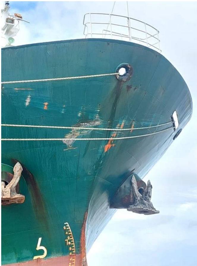
Image 4 - Damage to the starboard bow of the Tradewind Passion
